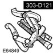
Remover, crankshaft seal 303-D121
